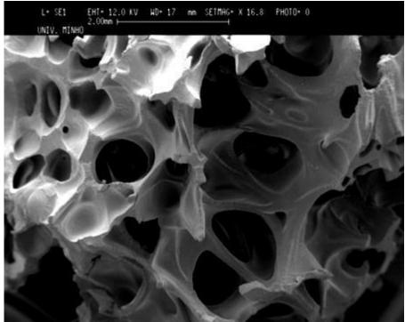
Figure 1.2- SPLA scaffolds processed by using a methodology based on extrusion with blowing agents.
