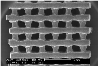
Figure 1.3- Scaffolds obtained by using rapid prototyping technologies: a) chitosan scaffolds processed by a 3D plotting methodology and b) PCL/PEG scaffolds obtained by Fused Deposition Modelling (Both images were a kind gift from Dr. Dietmar Hutmacher from the National University of Singapore).
