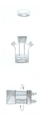
Figure 4- Bioreactors types used in the bone tissue engineering field: a) static; b) spinner flask and c) rotating wall vessel reactors (adapted from [46]).
